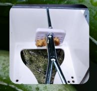
Mount the base approximately 1 metre from the ground, using the nails and screw provided. We recommend removing the steel frame, to make mounting the base easier.
